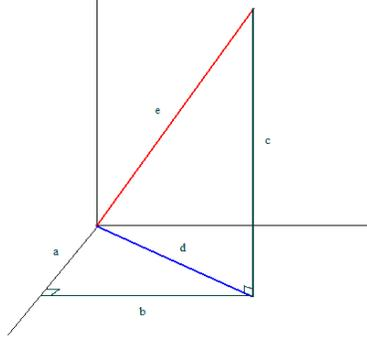
Figure 2: Length of vector in three dimensions
